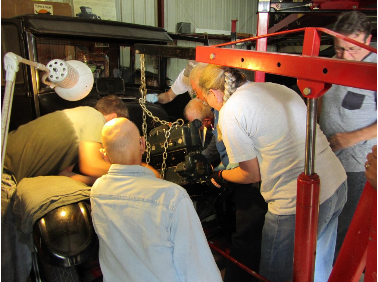
Rueben & Don were inside the car to guide the transmission and pedals past the firewall.
