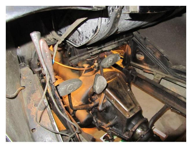
With plenty of willing hands to run the jack and position the engine, the crew pulled the engine forward on the disconnected rear engine mounts. The mounts conveniently slide along the frame rails. Once forward enough, the hoist did the hard work while we steadied and slightly turned the engine with Dan's direction in order for the pedals to clear the firewall.
