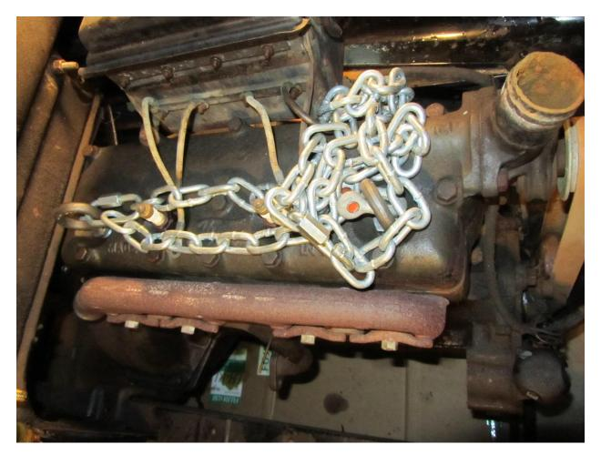
We adjusted the chain to give the estimated angle for "up-and-out" hoisting of the engine and transmission. Since the three control pedals stay attached to the transmission, Dan Baxter worked from inside the cabin to make sure the pedals cleared the firewall through the access hole.
