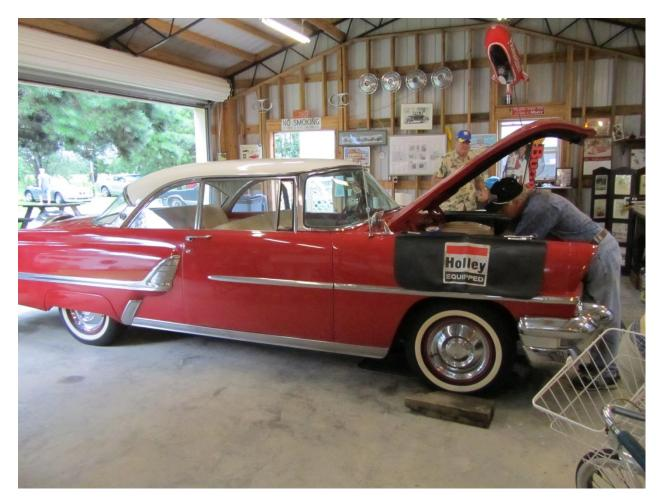
By 0900 Bill O'Rourke's garage was open and Bill B. was extracting spark plugs to do a compression test. The original theory was the stumble could be caused by a sticking valve or improper valve clearance. A compression test would quickly show if a valve was sticking open and a read of the spark plugs could yield additional clues.
