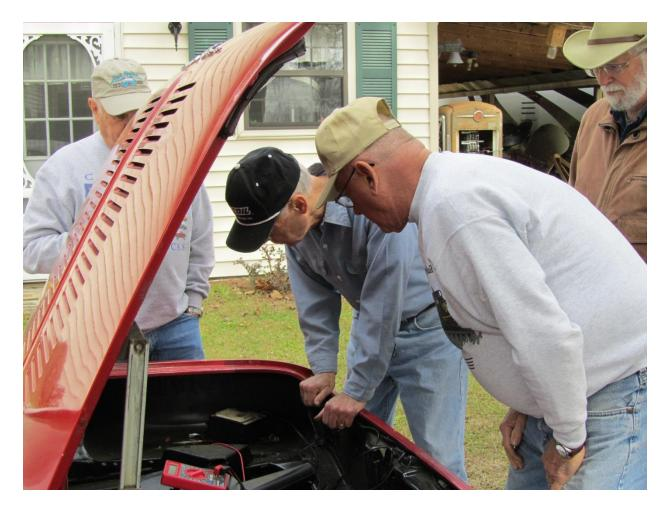
The distributor cap was removed and the points checked out. A dwell meter was hooked up and the dwell checked out with the hot wire in place to allow the engine to start. The battery was then charged to full capacity just to make sure it was up to the task. The Corvair still would not crank without the hot wire in place.
