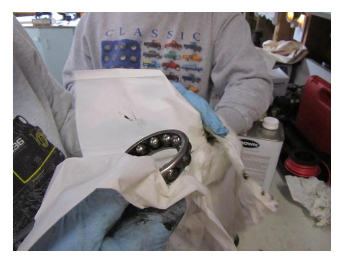
We were able to read a clear part number off the inner bearing race and Bill O. began making his parts needed list. A trip to NAPA would be required to order the correct parts. The crew celebrated the accurate diagnosis and verification of that diagnosis with coffee and donuts.
