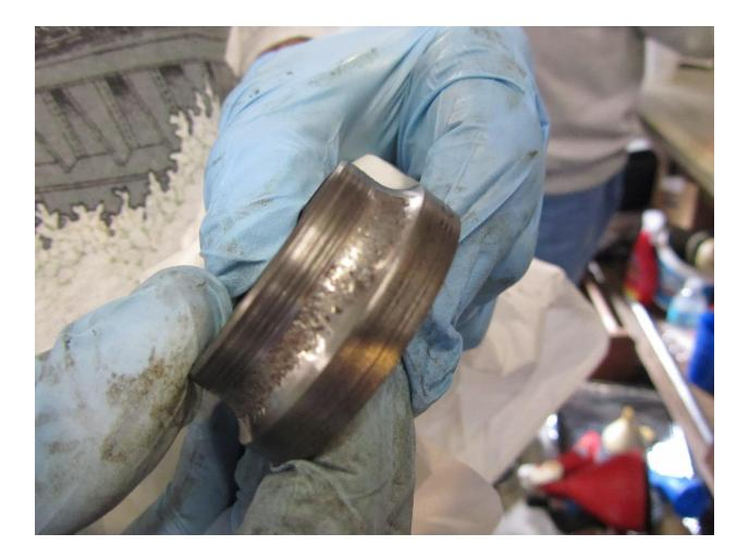
As the bearings were lifted out of the hub for inspection, the Model A owners began to get excited. The 1959 Chevy had been riding around on round ball bearings just like the Fords from the 1930s! No fancy taper roller thrust bearings needed here—if it was good enough for granddad, it's good enough for us. The outer bearings and races were in very good condition, the inner bearings had taken all the wear-and-tear.
