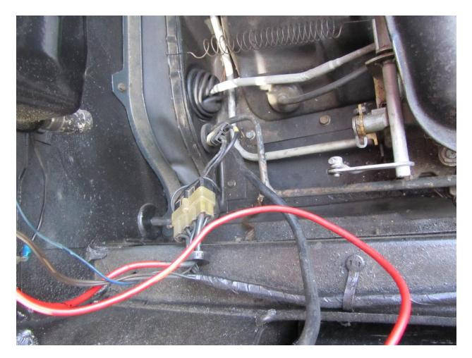
Bill O. promised to pick up some contact cleaner at NAPA and do a proper cleaning of the connector. We are confident this will result in a proper 12 volts making it to the coil and the Corvair should be back to consistent cranking.
