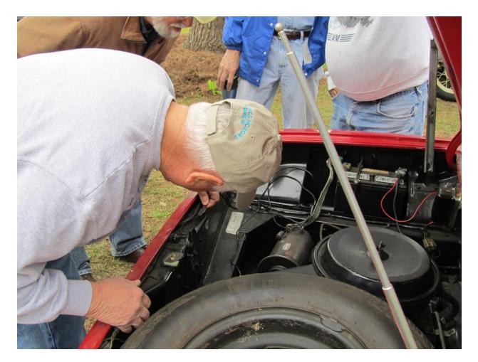
A jumper wire, or 'hot wire' as known by the former juvenile delinquents in the group, was attached from the battery to the hot side of the coil. This allowed the Corvair to start and run just fine. Something was happening in the wiring, connectors or ignition switch to starve the ignition circuit of vital electrons.
