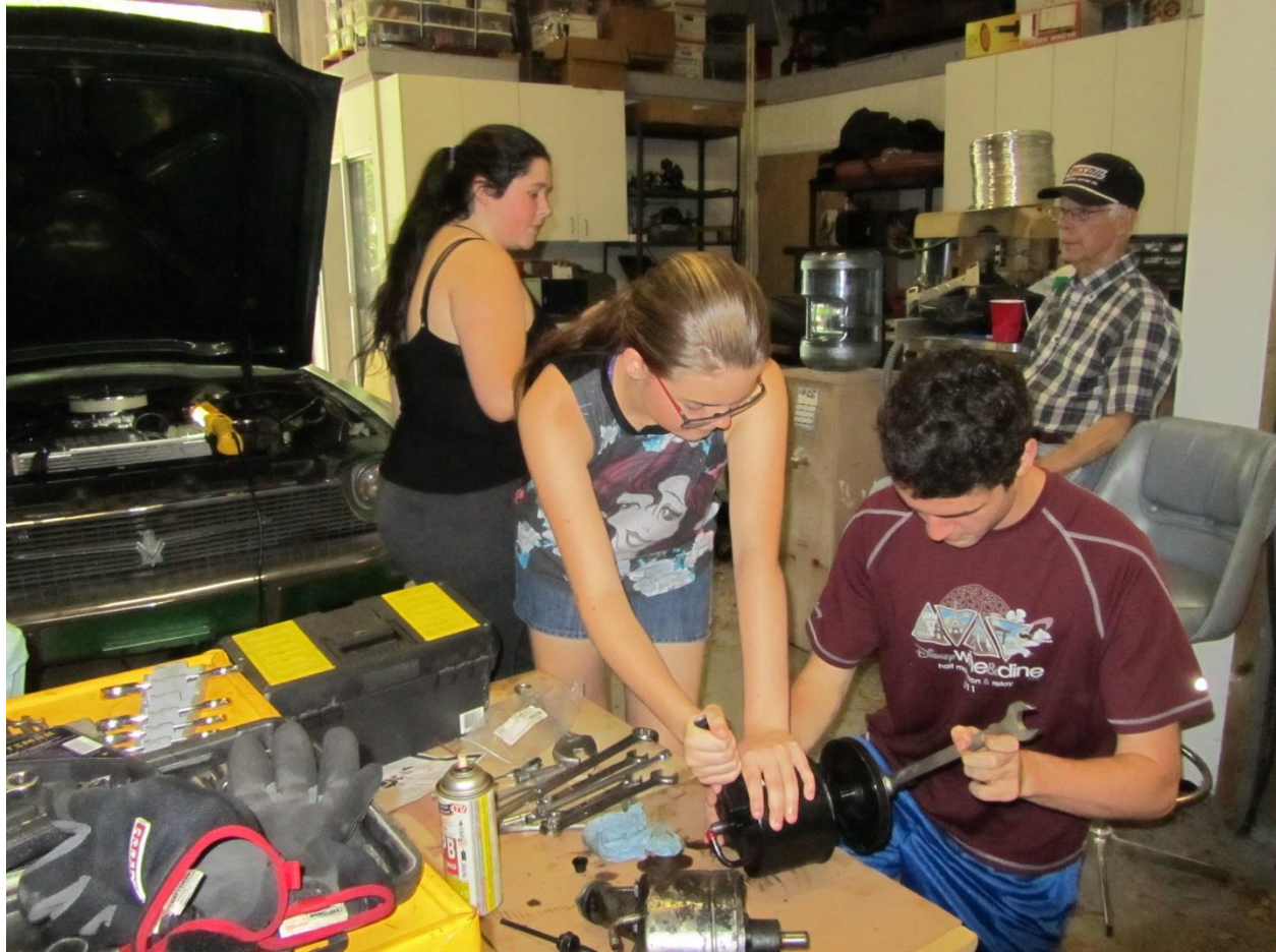
When break time and story time ended, Sloane, Ariana and Seth used the pulley installation tool to press the pulley onto the rebuilt pump.
