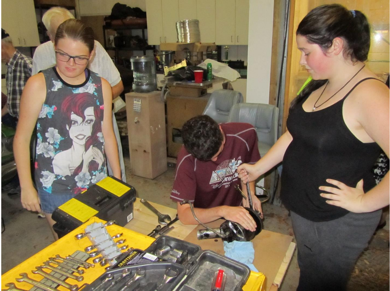
Ariana, Seth and Sloane assembled the puller and soon had the pulley off the old pump. This was set aside to be used on the rebuilt pump.
