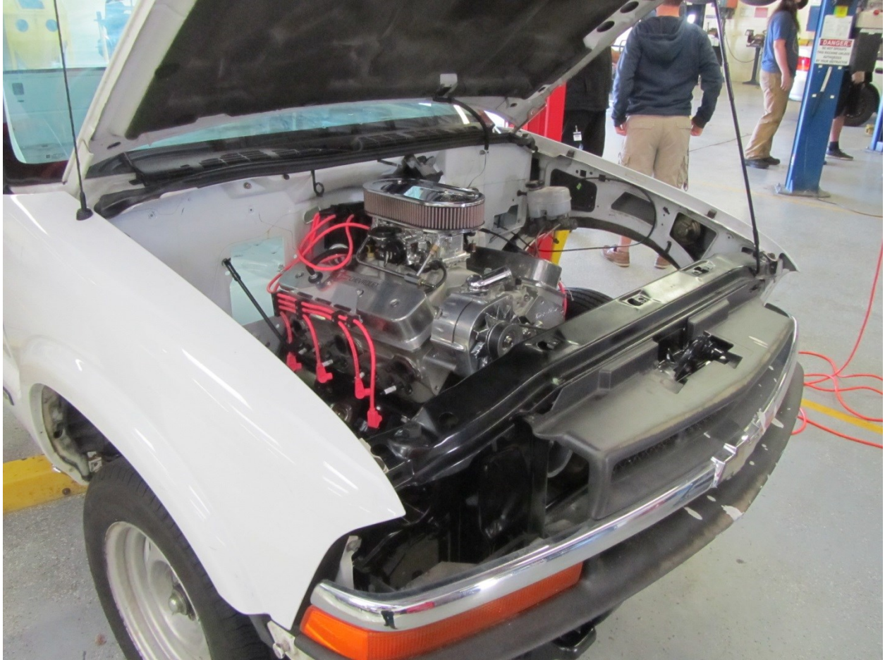
Race truck powered by a modified Chevrolet 350 engine and using a four-link rear suspension to improve traction and handling
