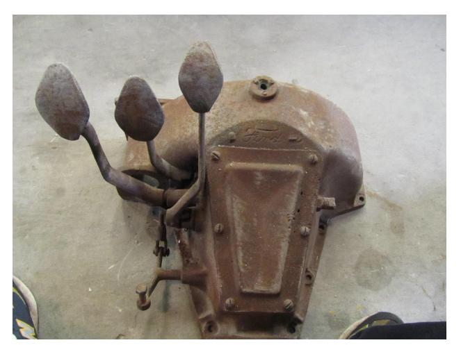
Those with wide feet were shown how to rotate the ankle and use the blade of the foot to depress the reverse pedal in the middle without pressing the other two pedals. This is sort of the antithesis of performance driving heel-toe technique.
