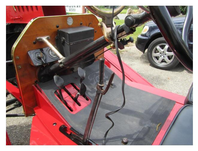
Norm also covered proper use of the choke and showed some Model T modifications such as front oil feed to increase main bearing life and a water pump. After all questions were answered and all fears allayed, the next step was the high-tech Model T simulator to allow student drivers to master pedal coordination.
