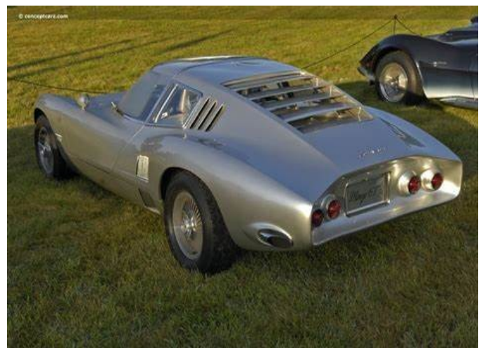
Rear view showing the sculpted taillight area, and electrically operated rear window louvers.
