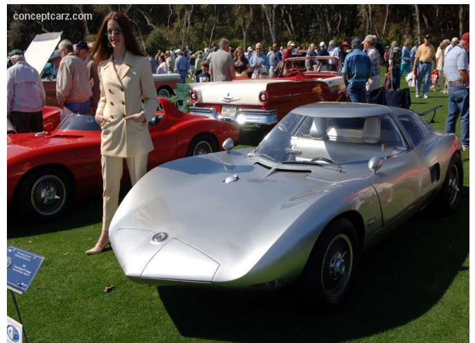
Left front showing the clamshell headlight covers. They opened electrically and added to the streamlined look.
